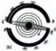
Bimetallic Strip for Thermostats & Clocks
