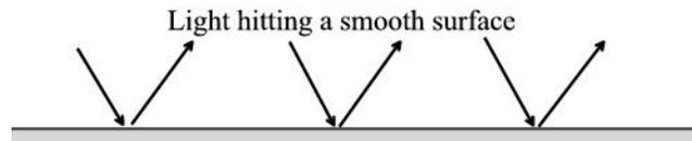
Light coming from a light source is called an incident ray and the light that bounces off the surface is called a reflected ray. A line that is perpendicular (90°) to the plane mirror is called the normal line. The angle between the incident ray and the normal line is called the angle of incidence ( $i$ ). The angle between the reflected ray and the normal line is called the angle of reflection ( $r$ ).
