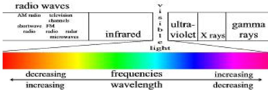
Different colors on the electromagnetic spectrum have different wavelengths (nanometers) and different frequencies (hertz).
