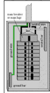
Each **branch circuit** is connected in parallel to wall plugs, lights and wall switches within a particular area of the house.
