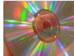
The rainbow spectra that can be observed on a CD are produced because the grooves on a CD act as a diffraction grating.
