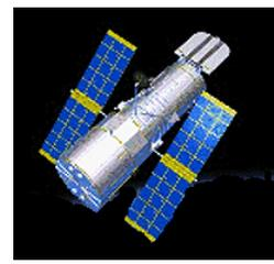
To improve the views of space, astronomers are able to access images from a telescope in space. Free from the interferences of weather, clouds humidity and even high winds, the **Hubble Space Telescope**, launched in 1990, orbits 600 kms above the Earth, collecting images of extremely distant objects. It is a cylindrical reflecting telescope, 13 m long and 4.3 m in diameter. It is **modular** (parts can be removed and replaced) and is serviced by shuttle astronauts.
