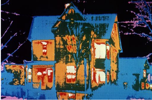
Infrared image of where heat is lost in a building
