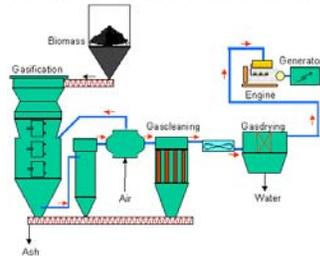
**Biomass**, solid material from living things, is also burned to power these thermo-electric generators.
