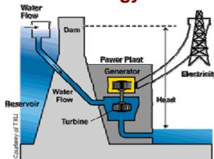
**Hydro-electric** plants use falling water (gravity), and pressure to generate electricity. Large dams raise the water above the power plant (which is usually built inside the dam), near the base.
